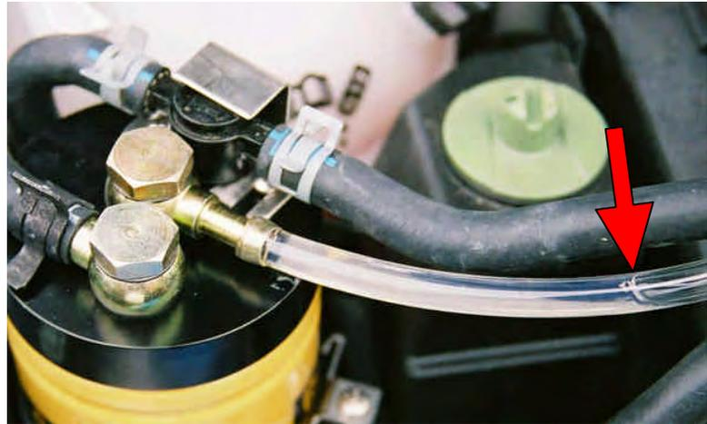
21. Connect the fuel line which feeds the engine to the filter outlet banjo fitting.
