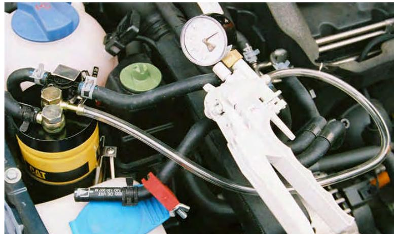
20. (Optional) Once you see diesel fuel in the vacuum hose, remove the vacuum and disconnect the hose. The filter is now primed.
