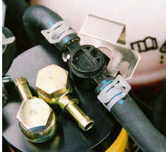
17. Twist the tee to expose the bracket screws below the tee. Tighten the screw, then twist the tee the other way to tighten the other screw.
