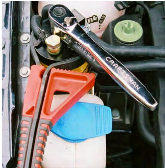
23. Adjust the filter in the holder to make sure that it is not touching the A/C line below it. Push the filter down until it touches the A/C line, then lift it back up approximately 1/4".
