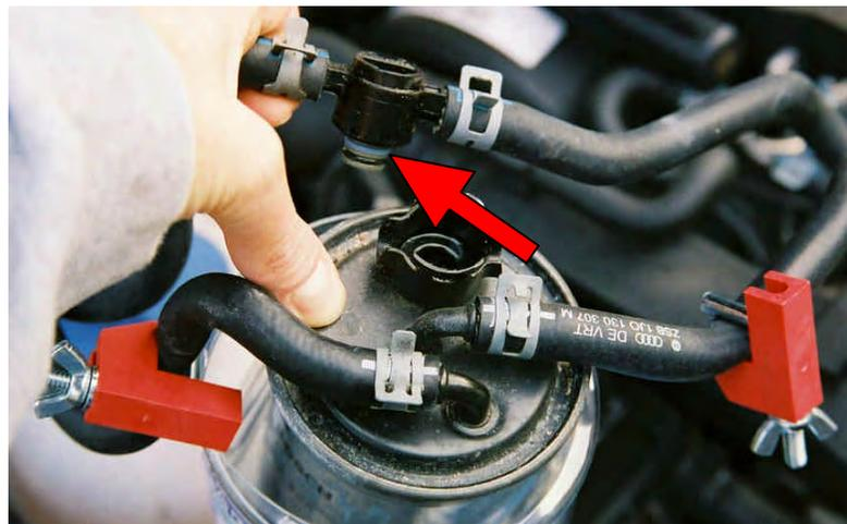
11. Remove the old filter and dispose of properly.
