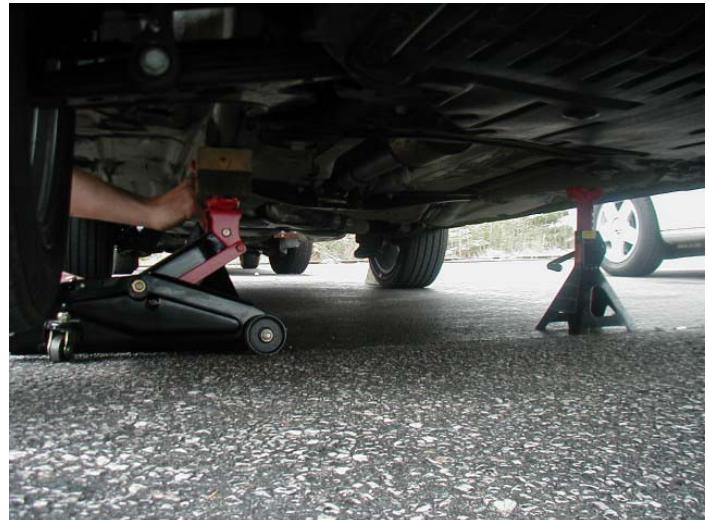
3. In my personal experience, I have found that with my rolling jack, if I put a 4" wooden block on top, not only do I get extra lift, but I protect the lift point from damage from the jack. Just be careful not to have the car slide off the jack.
